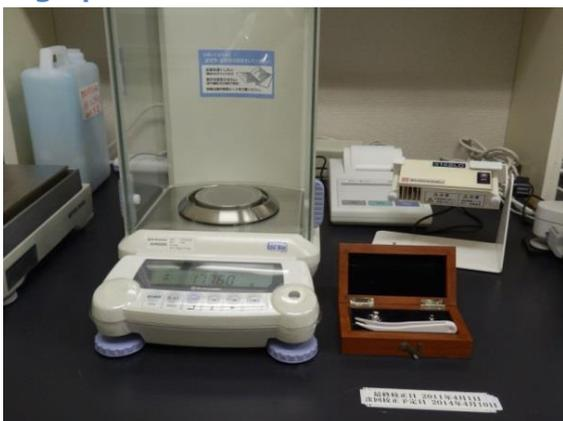
The balance, which can certainly measure to 0.1mg, is placed on an aseismic plate where it is not affected by static electricity, nor subtle vibration.
