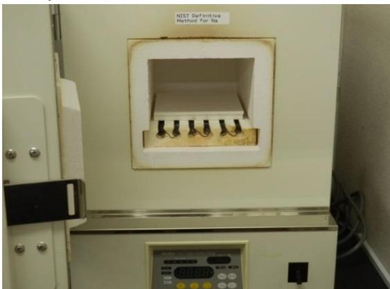
The picture above shows a high performance furnace used for decomposition of protein in serum for analyzing the amount of Na and K in a serum sample.
