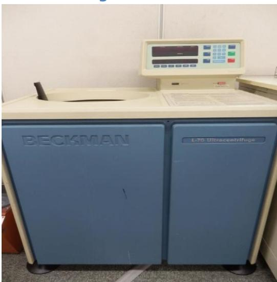
A Beckman Ultracentrifuge, shown above, is an essential instrument for performing the BQ method developed by the Centers for Disease Control and Prevention (CDC). The laboratory of ReCCS is equipped with swing rotors and angle rotors, necessary for the separation of lipoproteins by ultracentrifugation according to the Hatch and Lees protocol.
