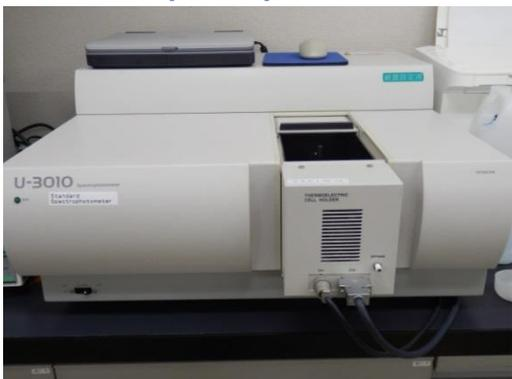
A molar absorbance coefficient is applied for the Cyanomethemoglobin method defined by the International Council for Standardization in Hematology (ICSH). Therefore, traceability of precise values of temperature, cuvette length(10.0 mm), and wave length are prerequisite.
