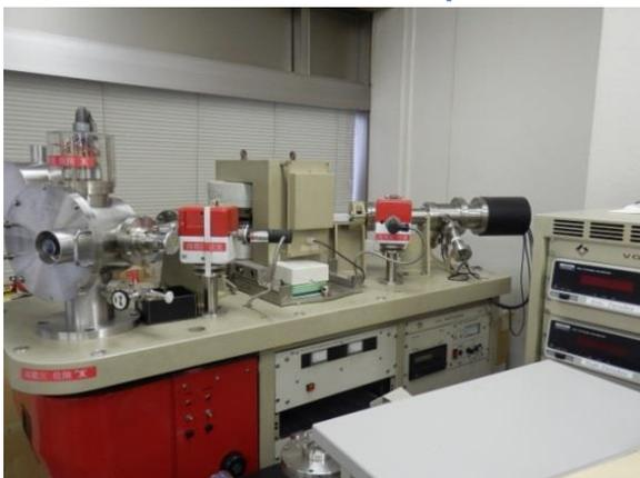
For measuring the amount of K in serum primary reference materials by an ion-selective electrode, thermal ionization mass spectrometry, which currently gives the highest possible accuracy, is used.
